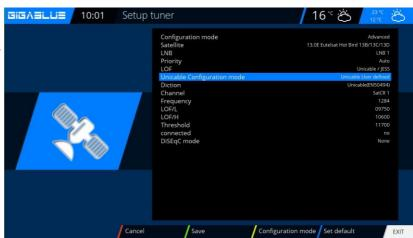
If more than one tuner available, so each tuner must be assigned its own channel
